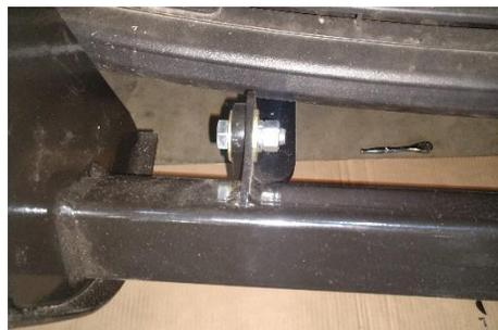
18. Separate the bumper skin and the lower splash shield to reach in and tighten the bolts on the lower mount.
