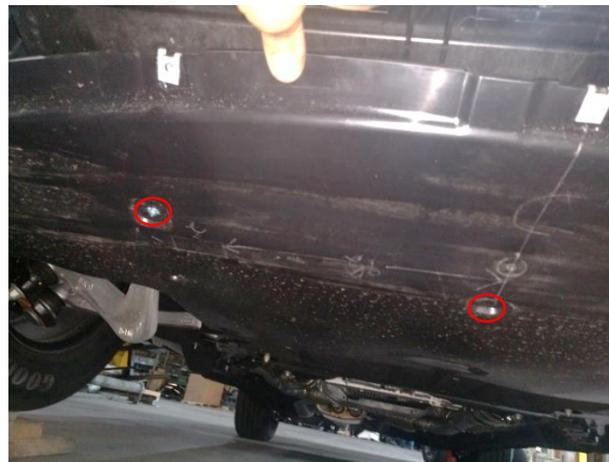
13. Remove the two 13mm bolts that are shown in the photo below. Right below the bolts that were just removed, cut a 1/2 x 1" slot to allow the lower mount to pass through.
