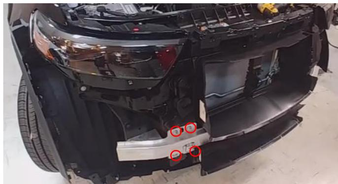
10. Start the tow lug of the aluminum bumper into the square cutout of the TS upper mount and rotate the bumper into place. Align the perimeter of the square mounting pads of the TS upper mount and the aluminum mount. Install the 3/8" hardware that is provided onto the TS mount and tighten completely.
