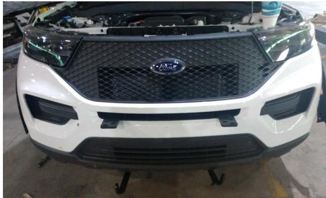
16. Set the grille guard on top of the upper mounts and start the six 1/2" provided bolts.
