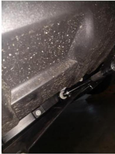
19. Tuck the splash shield above the bumper skin. Re-install all the bumper skin bolts and tighten.
