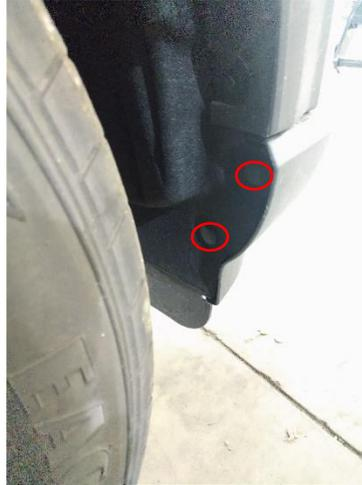
3. Remove the four 7mm bolts from the front of the inner wheel liner.
