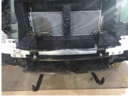
15. Re-install the bumper skin by clipping the grille section at the top. Do not install any bolts at this time.
