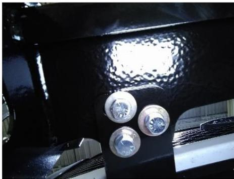
17. Attach the lower mount to the guard using the provided 1 1/2" hardware.
